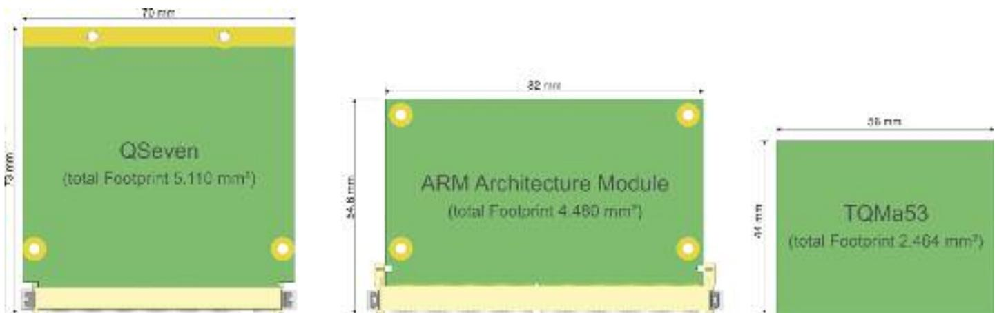
Figure 2: Q7-KARMA-TQMa53 comparison with plugs
