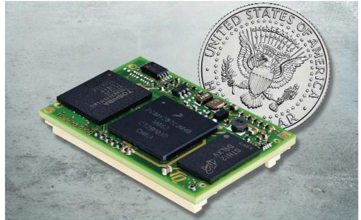
*In the TQMa28, TQ relies on proprietary technology in order to ensure that all the features of the Freescale i.MX28 can be used on the smallest possible space.*
