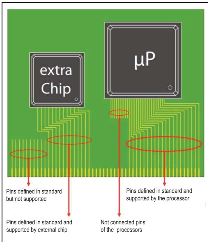
*Sometimes the chip fails to recognize a signal; sometimes the signal is not envisaged under the standard: standards, in view of the large variety of ARM processors, have their limits.*
